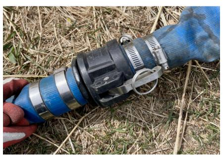
• Attach the 1 inch or 2 inch blue hose to the other end of the pump, secure by flipping both metal snaps down. Make it longer by attaching more hoses together, flip metal snaps
